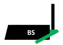
Optimize the signal for the front and upward Bend the TX antenna 90 degree upward and RX antenna 90 degree to sideward
