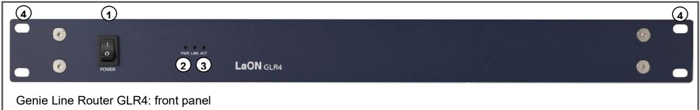
Genie Line Router GLR4: front panel
